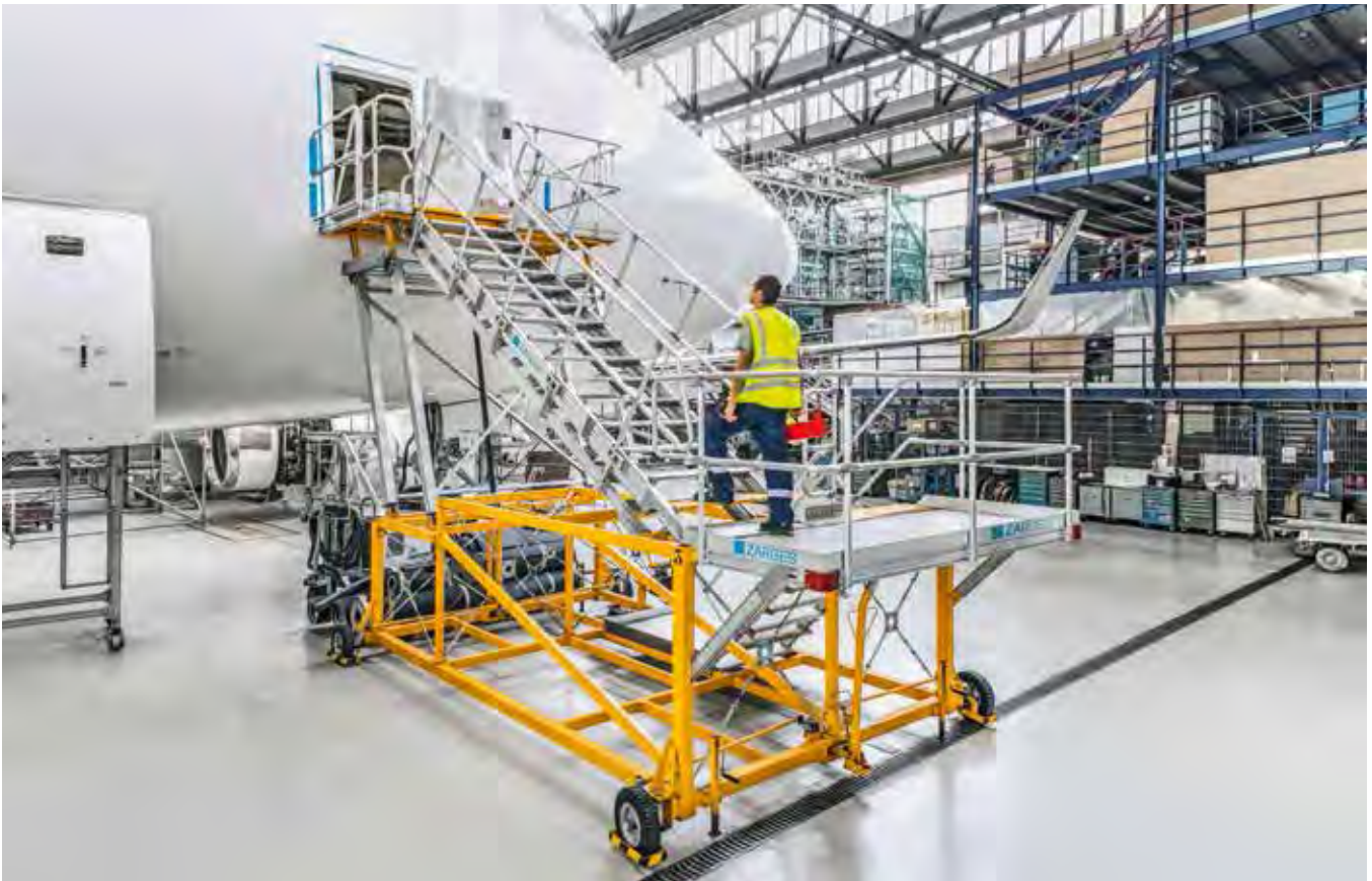
Maintenance stairs with with intermediate platform for working on passenger door access
