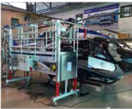
Maintenance platform with electrical height adjustment
