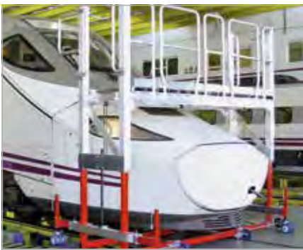
Height-adjustable front work platform with rail-guided chassis
