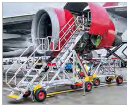
Engine stairs (UCAS). Narrow and brace-free designed for easier access
