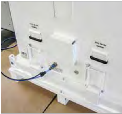
Water-vapour-proof container being leak-tested with overpressure
