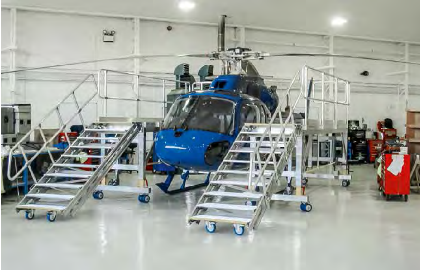
Height adjustable maintenance platform for an EC 145
