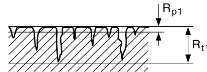
Surfaces produced by roller burnishing (cold formed surface)
