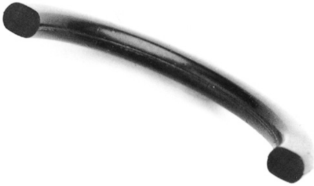
Fig. 10.8 Damage pattern caused by high compression set
