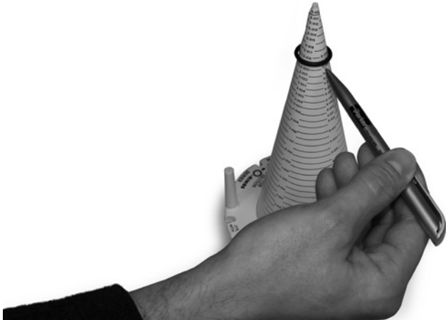
Fig. 5.8 Determination of the 2-xxx size number with the measuring cone
