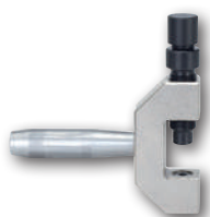
Husillo para remachar Riveting spindle
